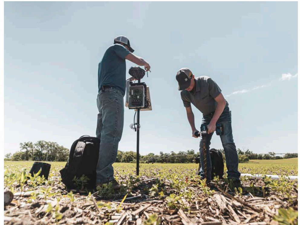
Soil moisture probe installation
