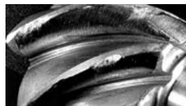
Gears run on competitive fluid shows wear and pitting damage
