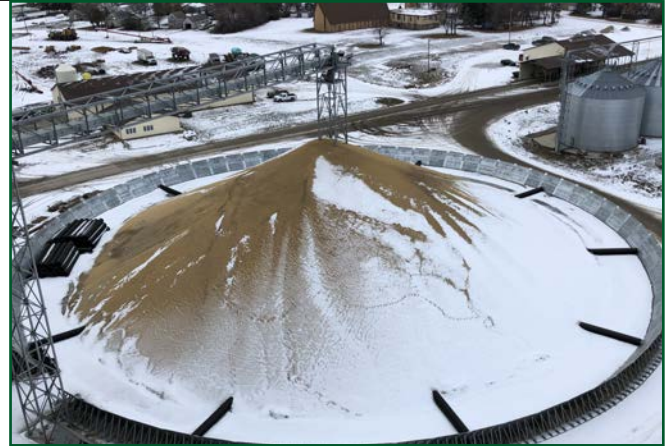
Soybeans stored (above) at Bisbee have since been picked up with no spoilage thanks to the member investment in the new concrete pad.
