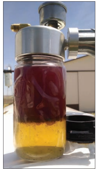
This sample shows water that has contaminated the tank.
